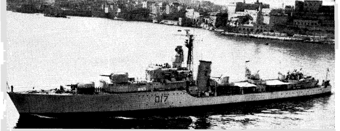
"Alamein," British destroyer of the "Battle" class, somewhat larger than vessels of the "Weapon" class. Outfitted as a destroyer leader when it was launched in 1945, it was scheduled for eventual conversion to radar picket service
