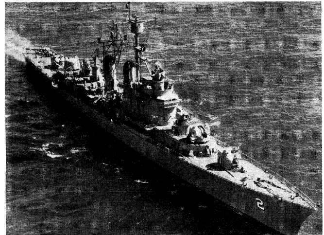
"Mitscher," U.S. navy destroyer leader (DL), officially rated as a frigate. The vessels of the "Mitscher" class are larger than some rated as light cruisers in other countries. The "Mitscher" was launched in 1952
