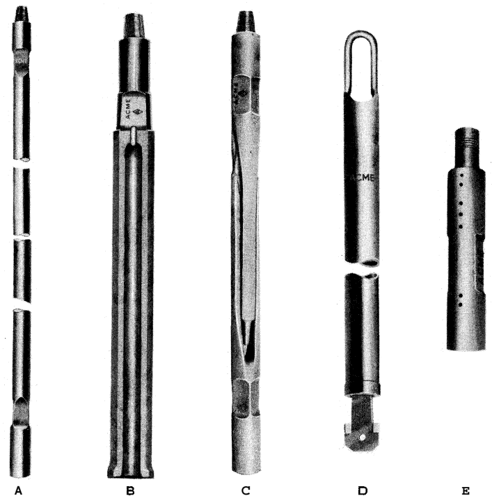
BY COURTESY OF ACME FISHING TOOL CO. FIG. 3.— DRILLING TOOLS (A) Drilling stem; (B) drilling bit; (C) drilling jars; (D) dart-valve bailer; (E) swivel socket for wire rope
