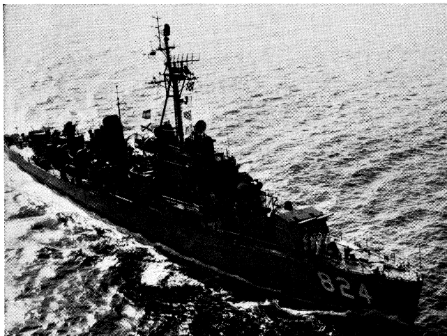
"Basilone," U.S. navy escort destroyer (DDE) of the "Gearing" class. Launched as a destroyer (DD) in 1945, later converted for antisubmarine warfare and completed as an escort vessel in 1949
